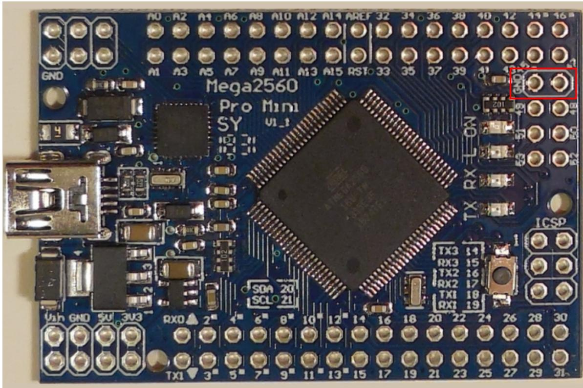
The wrong pinout will *still* work, *technically* - but would require manually running jumper wires between the boards, instead of using headers for installation.
